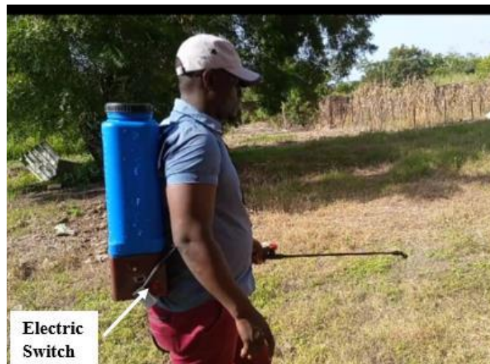
Plate 2: Testing the novel Battery operated Knapsack sprayer
